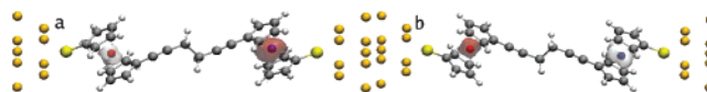
Figure 5. Charge difference of spin-up (a) and spin-down electrons (b) at 1.1 V between backward and forward scanning. White denotes electron loss, and red denotes electron gain.
